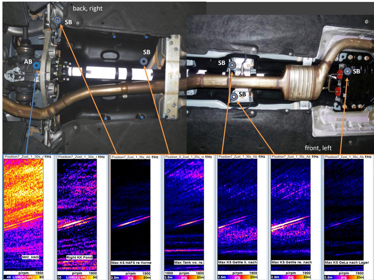
Fig. 7: Analysis of structure-borne sound with reference signals airborne sound
