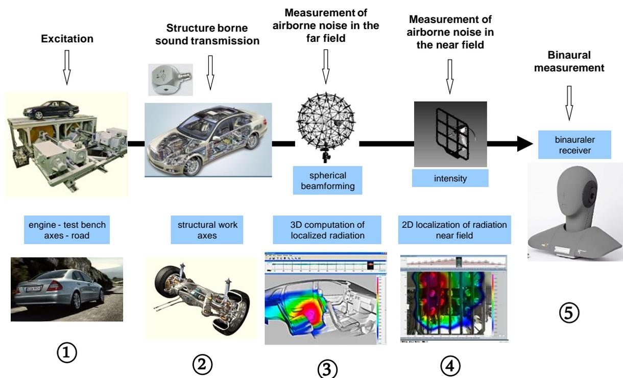
Fig. 1: Integral approach of source localization at Daimler AG
