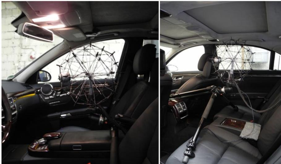
Fig. 3: Measurement positions of the spherical array in the vehicle cabine
