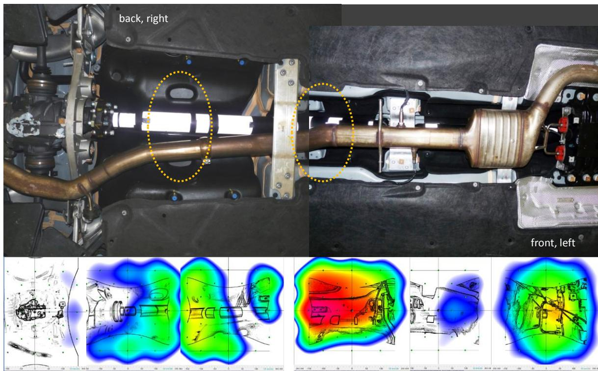
Fig. 8: Airborne noise emission of the cardan shaft detected with the Gfal intensity array
