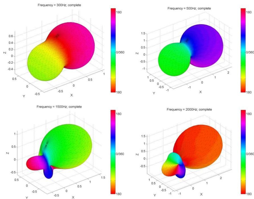
Fig. 4: Result of the plane-wave decomposition for the center speaker in the vehicle interior, Array position "Front"
