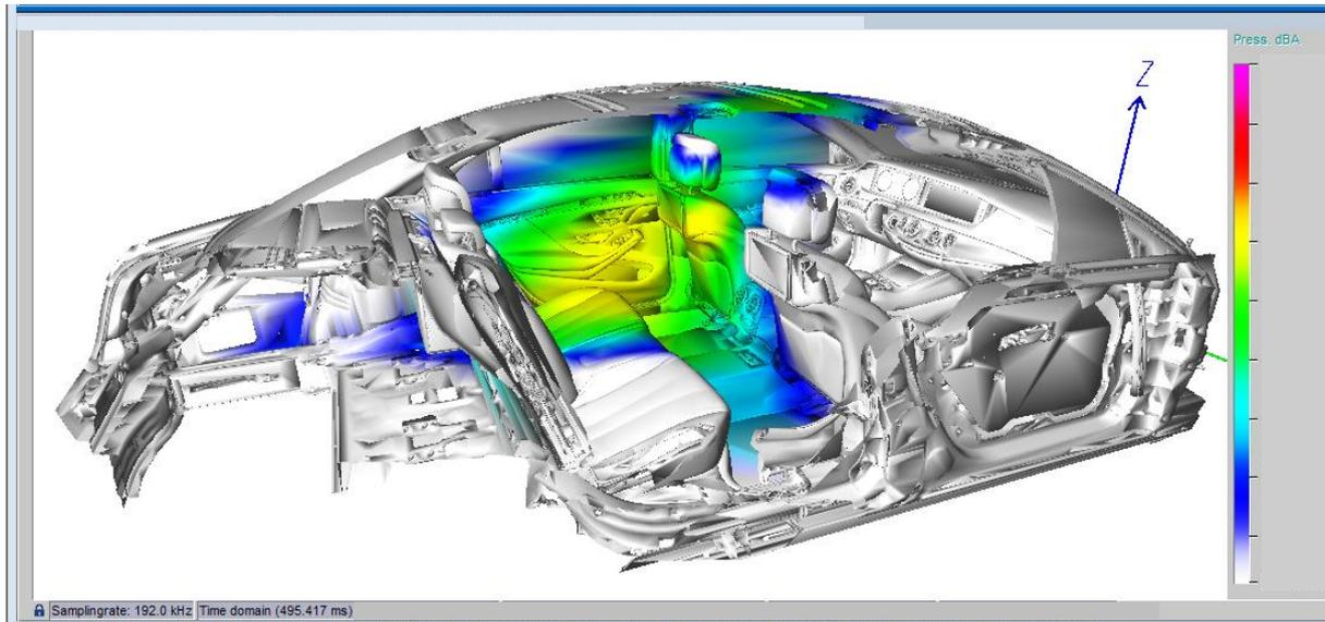
Fig. 9: Exemplary mapping of the sound field in the vehicle interior, SW: NoiseImage, GFaI
