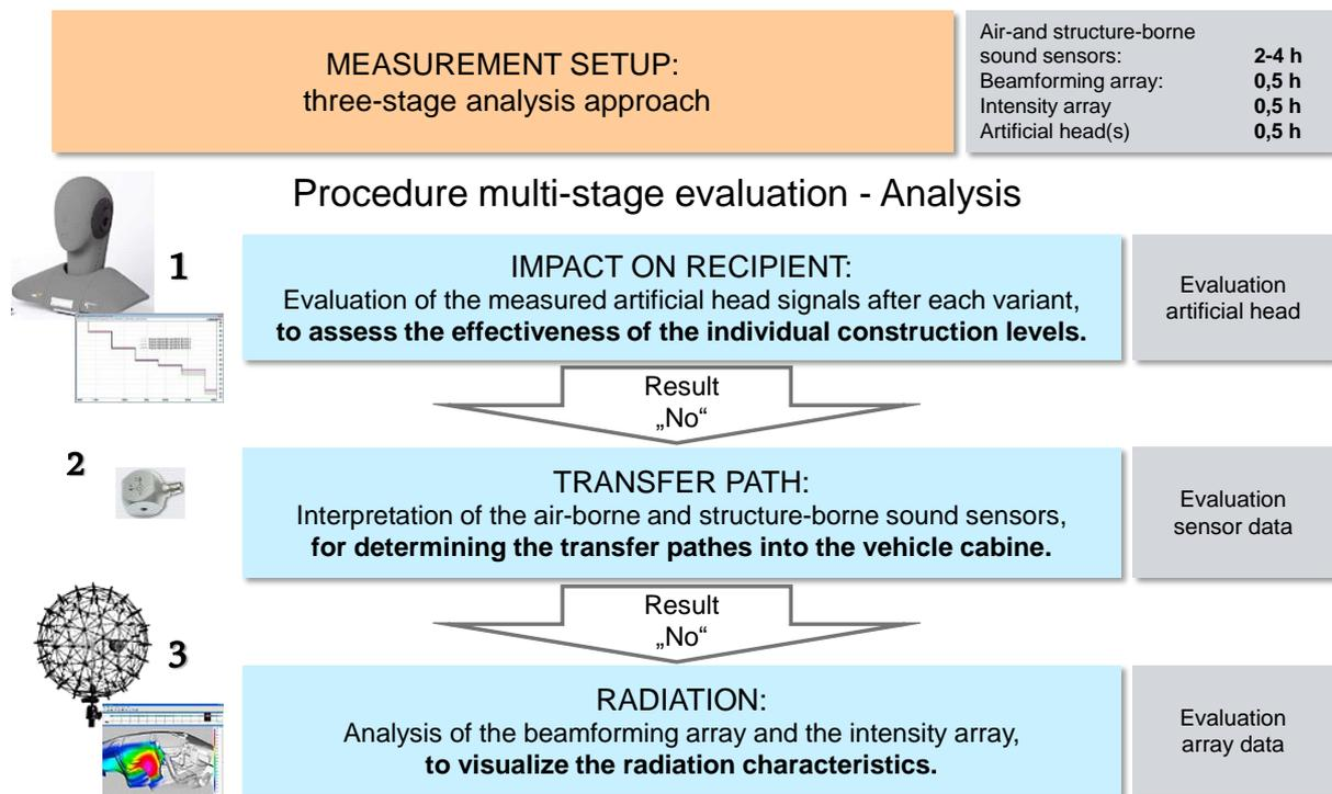
Fig. 2: Multi-stage approach of the measurement system “acoustic camera”
