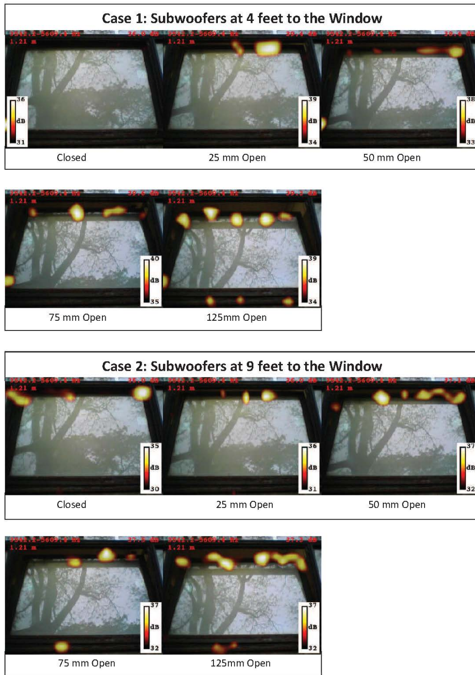
Fig. 11. Beamform maps using TIDY showing a comparison of the cases with speakers close and away from the window for the frequency range 3500 Hz – 5600 Hz for various window gaps.
