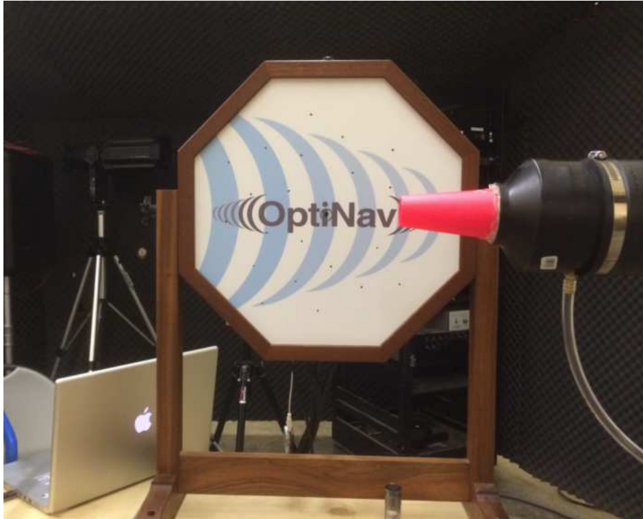
Fig. 1. Array 24 Jr set up for the jet noise test. The 24 microphones are arranged in a 0.35 m pattern. The jet speed is Mach 0.15.
