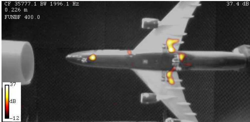
Fig. 16. Functional Beamforming of Airframe noise from a desk model of a Boeing 747-8. The spots near the leading edge of the wing root are from tiny depressions representing the air cycle machine inlets.
