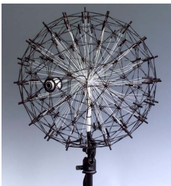
Figure 1: A sensor array consisting of 120 microphones placed regularly on a sphere of radius 60cm is combined with a standard CCD web-cam for acquiring an acoustical and an optical image simultaneously [3].
