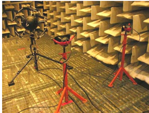
Figure 2- Measurements in anechoic room with different sources locations
