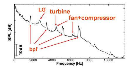
*Figure 3: De-Dopplerised spectra for a fly-over with extended landing gears for an emission* angle of  $\theta = 90^{\circ}$
