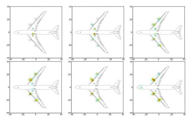
Figure 9: Results of the deconvolution analysis for a fly-over with extended landing gears from the high-frequency array;  $\theta = 90^{\circ}$ , 12 dB dynamic range, from left to right, top: 2500 Hz, 3150 Hz, and 4000 Hz; bottom: 5000 Hz, 6300 Hz, and 8000 Hz
