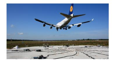
Figure 1: A Boeing 747-400 passing over a microphone array at Parchim airport (DLR, 2008)
