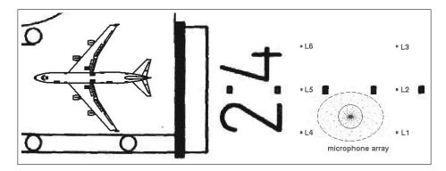
Figure 2: The set-up of the 42x35 m multi-arm spiral array for the B747-400 fly-over measurements of DLR and Lufthansa at Parchim airport, 2008; the aircraft on the runway is shown in order to indicate the relative size, the points L1–L6 mark the locations of the laser distance meters
