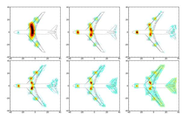
Figure 4: Results of the classical beamforming analysis for a fly-over with extended landing gears from the low-frequency array;  $\theta = 90^{\circ}$ , 10 dB dynamic range, from left to right, top: 200 Hz, 315 Hz, 400 Hz; bottom: 500 Hz, 630 Hz, and 800 Hz
