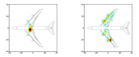
Figure 6: Results of the classical beamforming analysis for a fly-over with extended landing gears: left: tone in the 2500 Hz one-third-octave band; right: turbine tone in the 4420 Hz narrow band;  $\theta = 90^{\circ}$ , 10 dB dynamic range
