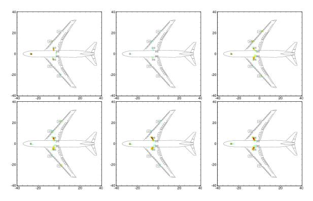
Figure 8: Results of the deconvolution analysis for a fly-over with extended landing gears from the lower frequency range;  $\theta = 90^{\circ}$ , 12 dB dynamic range, from left to right, top: 315 Hz, 400 Hz, and 500 Hz; bottom: 630 Hz, 800 Hz, and 1000 Hz
