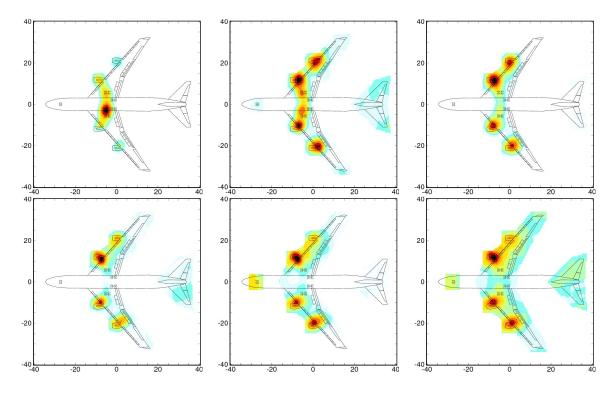
*Figure 7: Results of the classical beamforming analysis for a fly-over with extended landing gears from the high-frequency array; from left to right, top: 3150 Hz, 4000 Hz, and 5000 Hz; bottom: 6300 Hz, 8000 Hz, and 10000 Hz*
