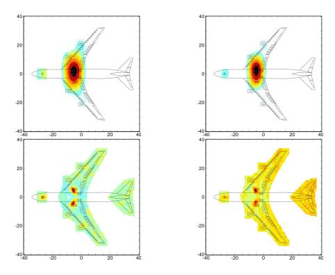
Figure 5: Results of the classical beamforming analysis for a fly-over with extended landing gears: overlap between the low- and the high-frequency arrays;  $\theta = 90^{\circ}$ , 10 dB dynamic range, left: 1000 Hz, right: 1250 Hz; top: high-frequency array, bottom: low-frequency array
