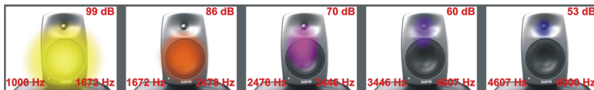
Figure 1: Multiband view of a two-way loudspeaker. Broadband noise with decreasing level to higher frequencies.
