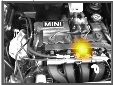
Figure 10: Noise radiation of the third cylinder in the 2-4 kHz frequency band.
