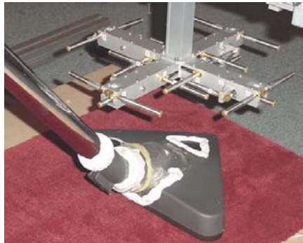
Figure 5: Test set-up of vacuum cleaner
